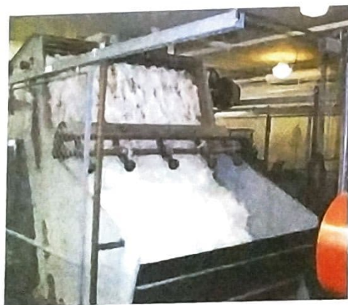
Fig. 3.5: Scouring in tanks
